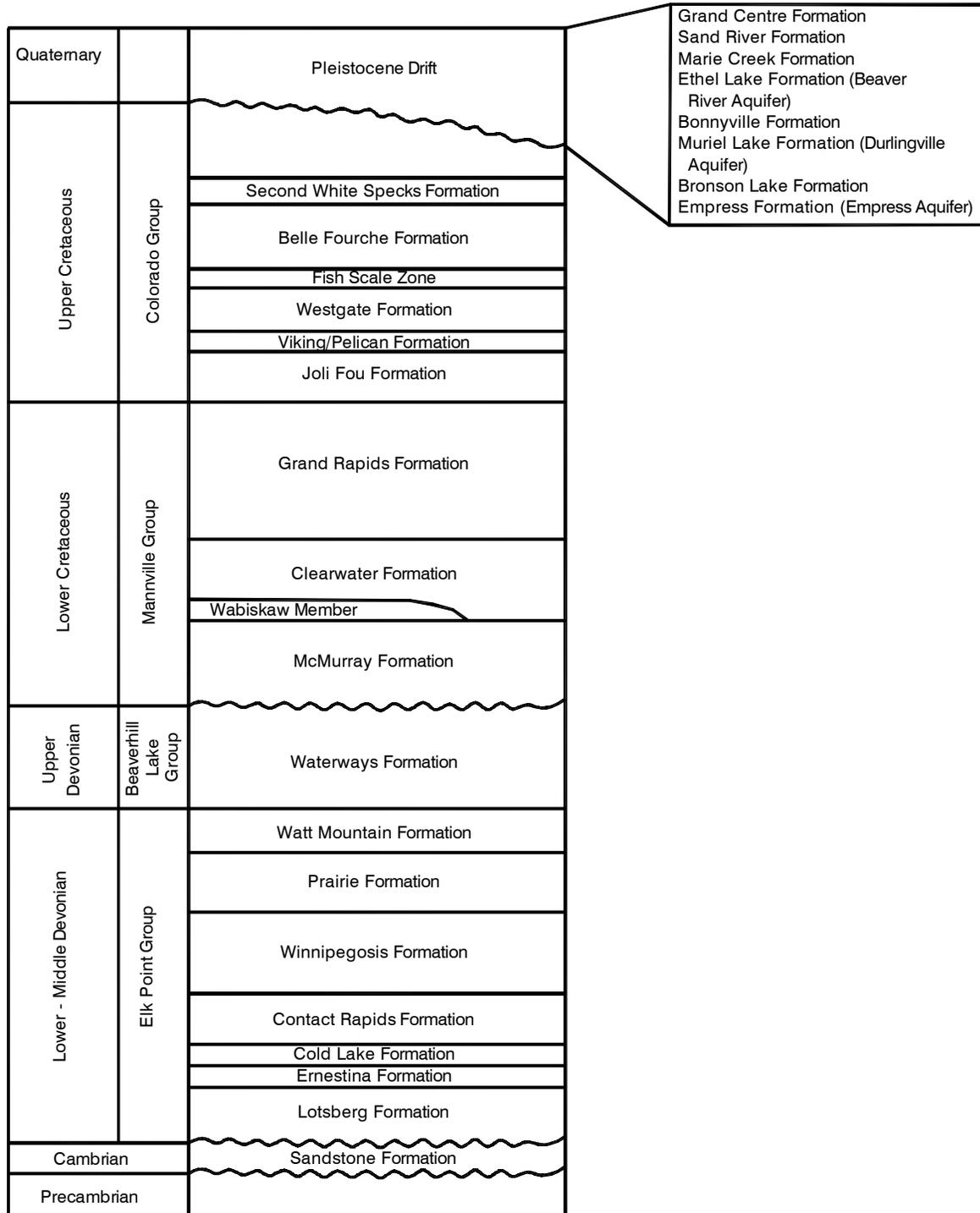
Figure 2. Cold Lake Expansion Project - Stratigraphy of the Cold Lake Area (Imperial Oil Resources Limited, Application No. 970163) (modified from Imperial Application, Volume 1, Figure 2-1)
