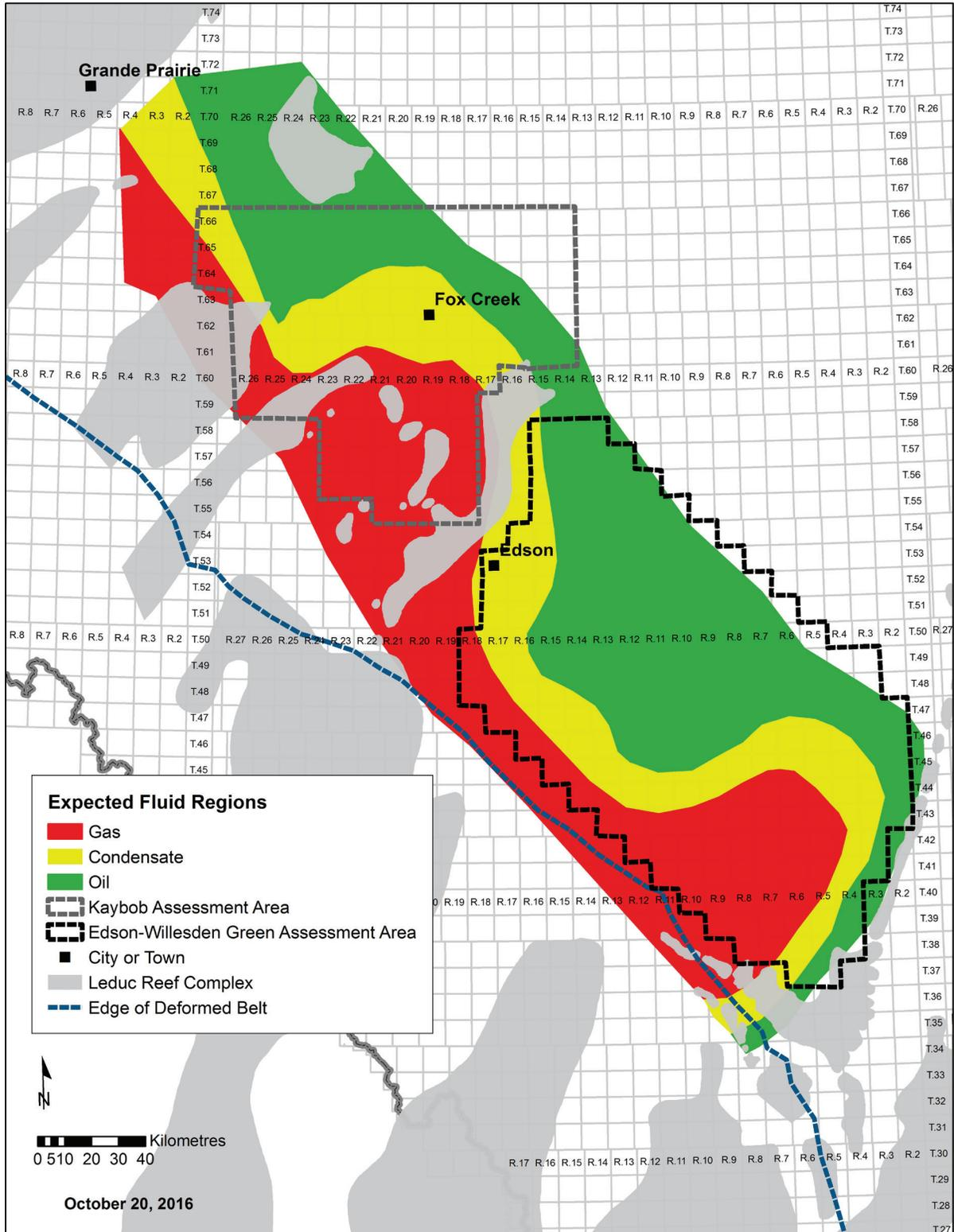
Figure 5. Expected fluid regions based on  $T_{max}$  analysis
