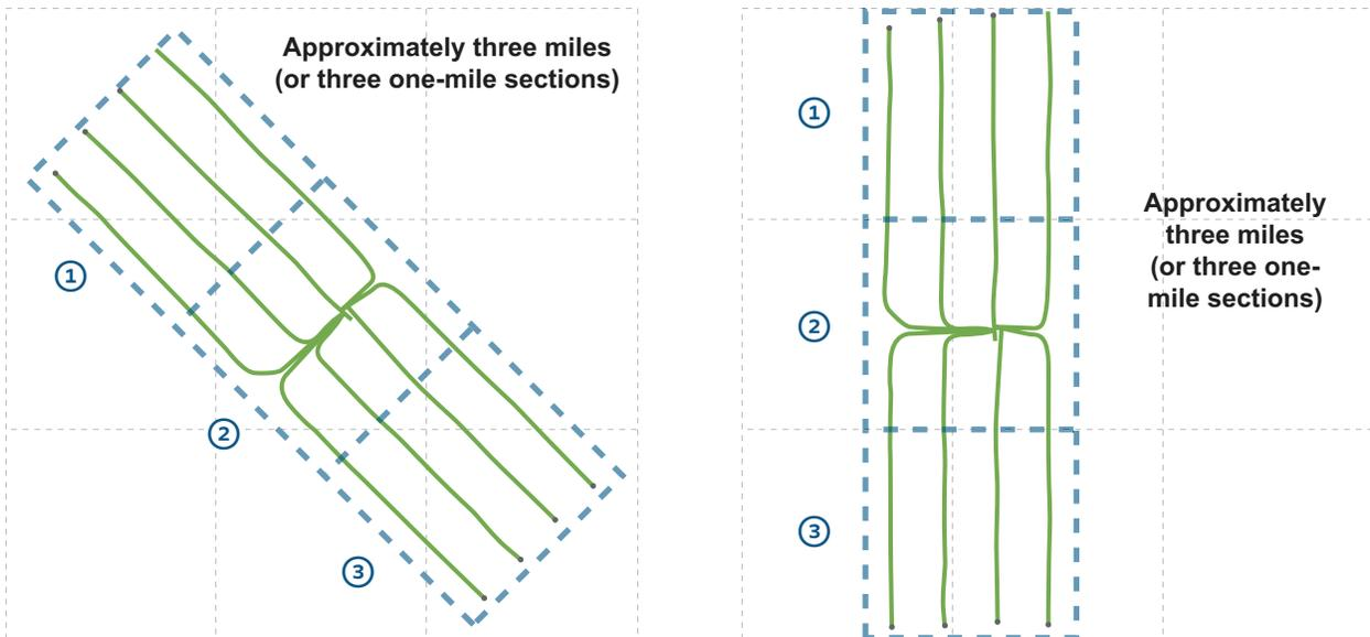
Figure 20. Eight-well pad configuration per three sections (8/3 rule)
