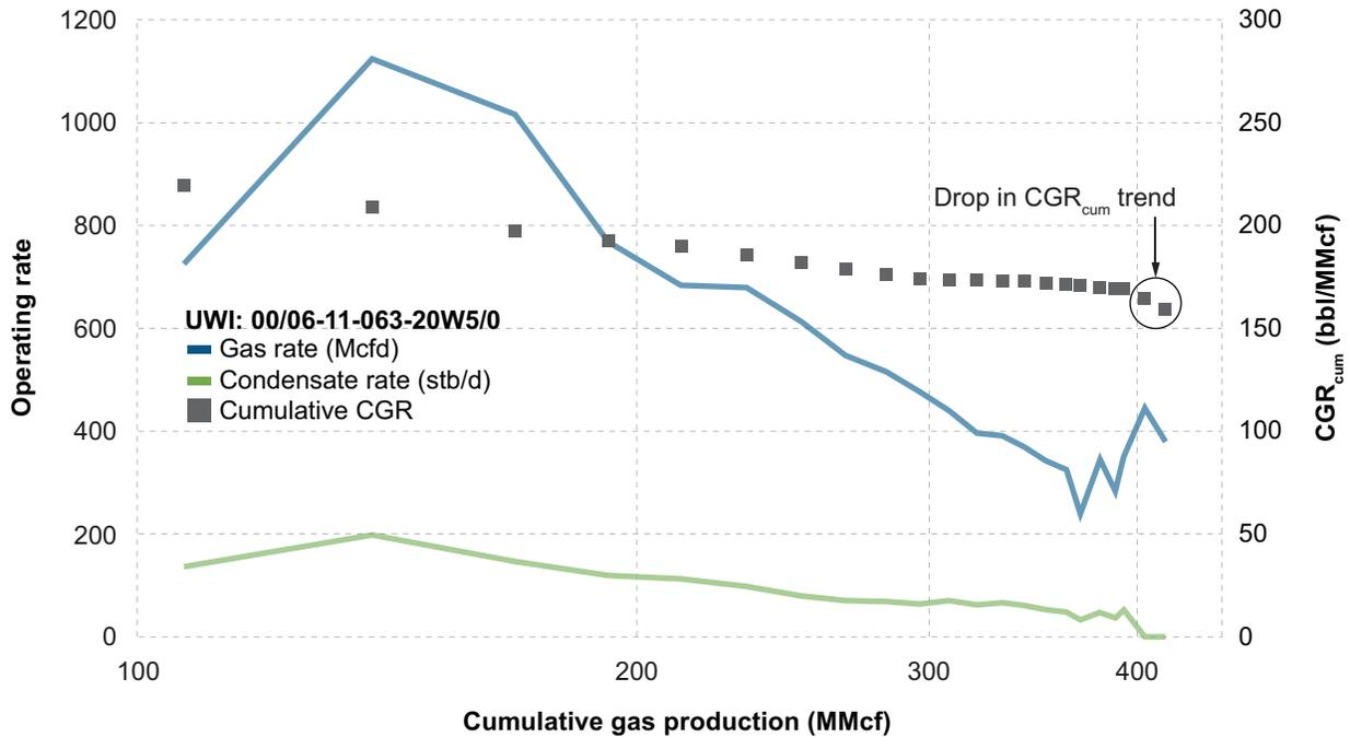
Figure 16.  $CGR_{cum}$  vs Cumulative gas production plot with secondary trends
