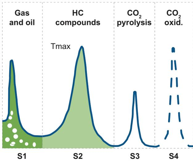
Figure 42. Hydrocarbon peaks measured from pyrolysis (from McCarthy et al., 2009)
