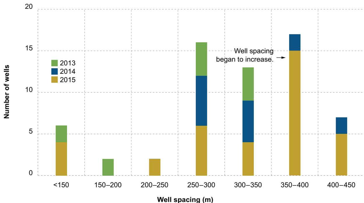
Figure 18. Kaybob pad well spacing by completion year
