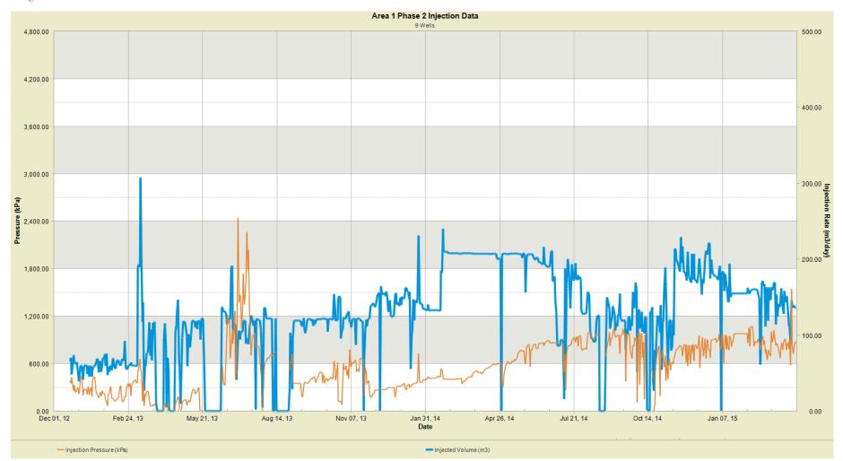
Mixed results with build up occurring on the 13-03 pad and conformance issues on the 4-10 pad
