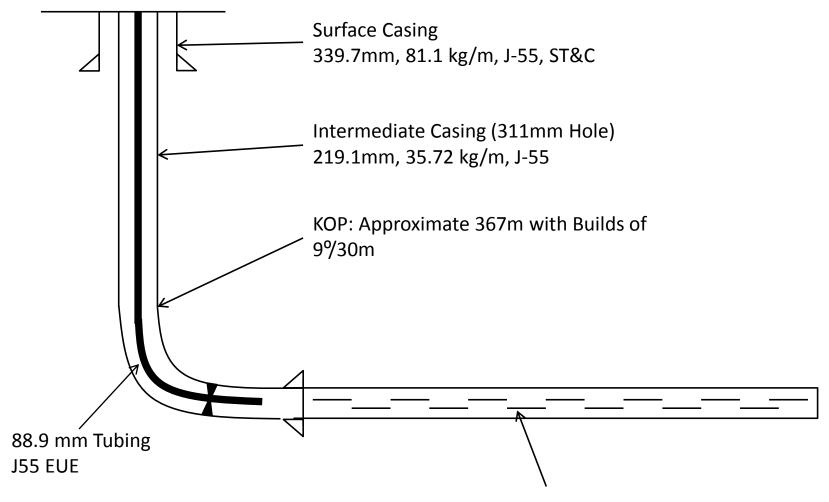
Slotted Production Liner (200mm Hole) 1600 m of 139.7mm,20.83 kg/m, J-55, ST&C
